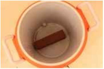
(650g brick into preheated cooler like so, pour boiling water on it)
